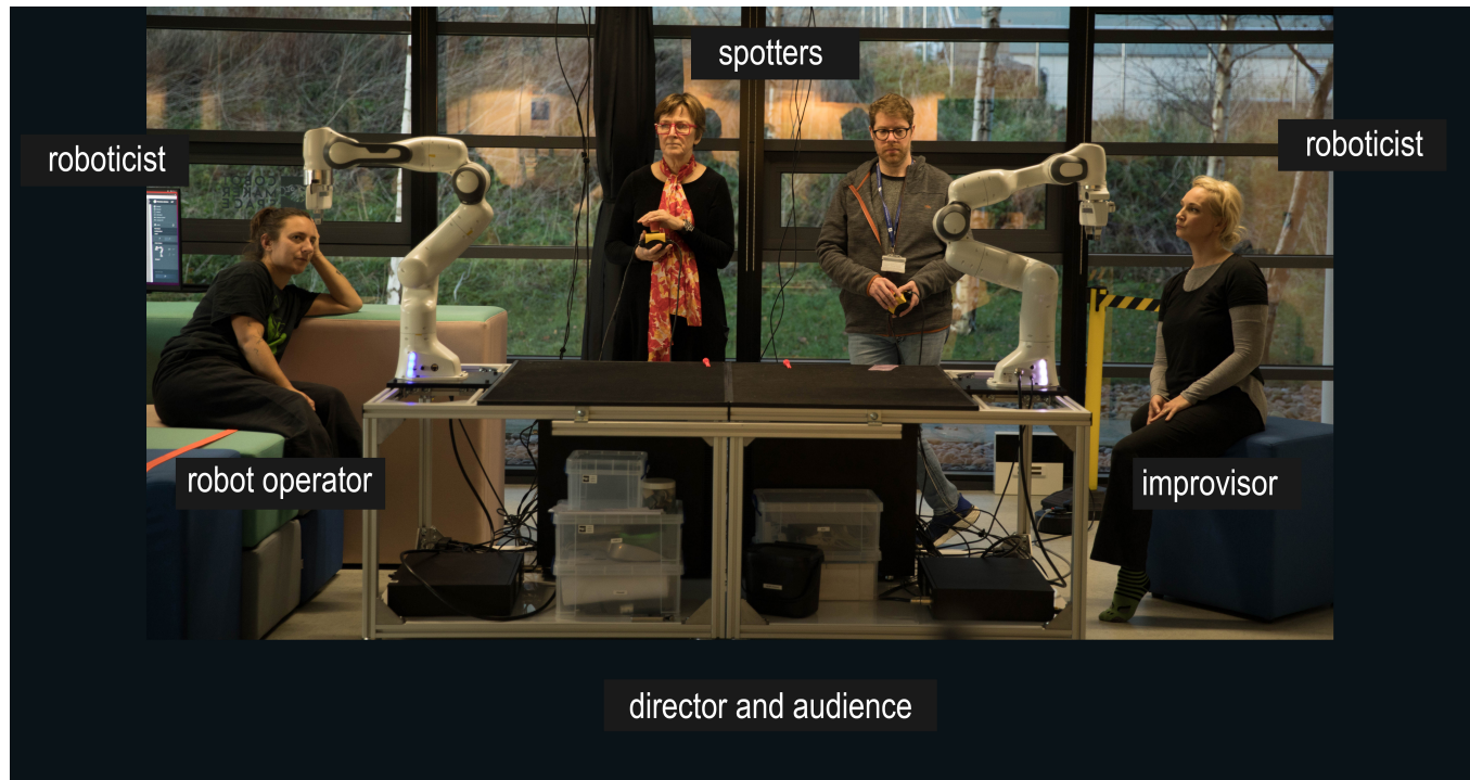
Figure 3: The safety setup: the dancer on the left operates the control arm while the dancer on the right improvises with the free arm. Each dancer is monitored by a roboticist near them. Two team members hold emergency stop buttons. The director and the audience are positioned behind the camera.
